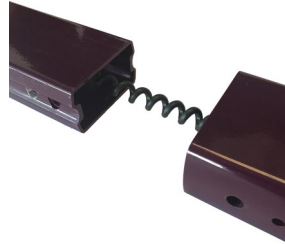
Figure 2. Sensor block/shaft interface
