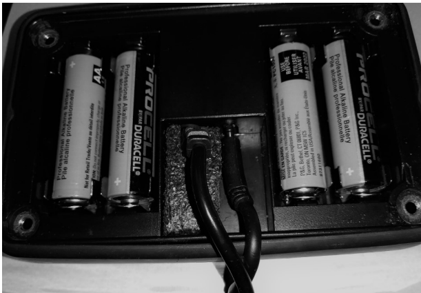
Fig. 1: Cable attached. Foam retainer installed
