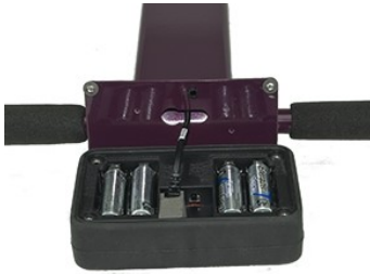
Figure 1. Sensor cable connection to board.
