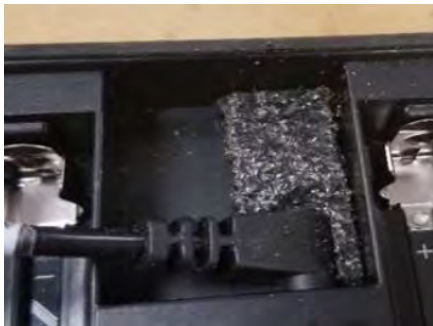
Fig. 2: Foam plug installed
