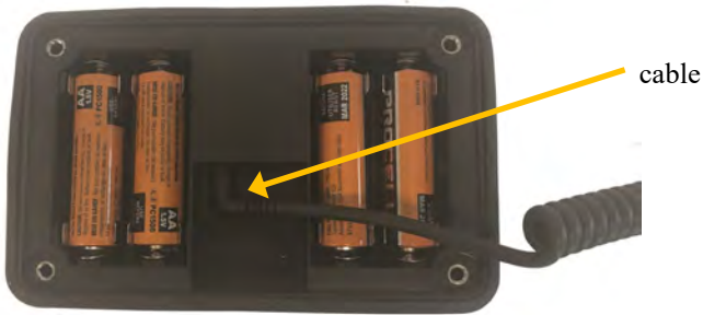
Fig. 1: Sensor Cable attached.
