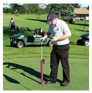
Lift plunger straight up to top of travel. Use foot support to stabilize the unit.
