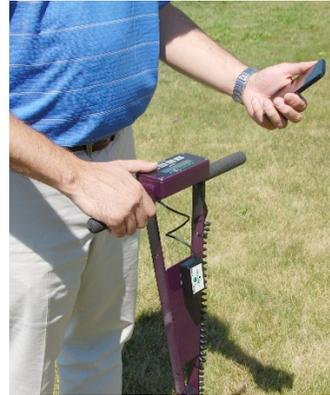
The FieldScout Bluetooth Device shown above (item 6453BT) connects to the data port of the TDR 300 meter. The TDR 300 meter must be using firmware version 6.5 or higher in order for the Bluetooth Device to work with a TDR 300 meter.
