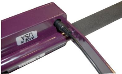
Image shows FieldScout Bluetooth Device plugged into the data port on TDR 300.
