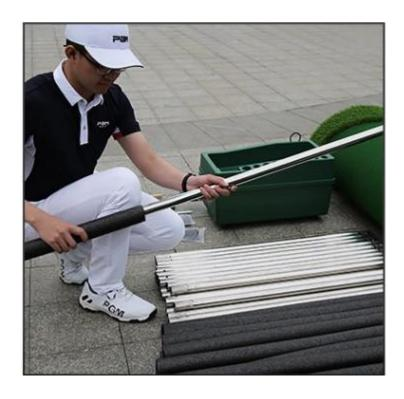
•Step 2: Insert steel tubes into the EPE tubes
